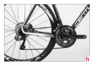
Shift carefully to the largest (inmost) sprocket (f) and check whether the teeth of the sprocket and the teeth of the guide pulley are all in a perfectly vertical line. Turn the limit screw marked "L" clockwise until the rear derailleur stops moving towards the spokes and can neither be moved by actuating the shift lever nor by pushing it with your hand (g). Carefully turn the cranks while checking.
